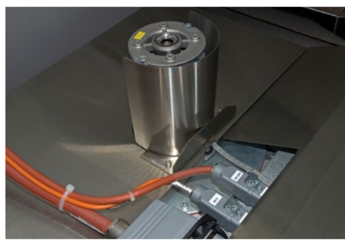
Recipe driven forced convection fan speed control
