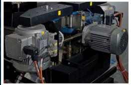
Reliable frequency inverter driven motors
